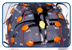
g.Nautilus is available with 32, 16 or 8 channels. Besides the gel-based active electrodes, also a version with active dry electrodes (patented g.SAHARA-technology) is available.
