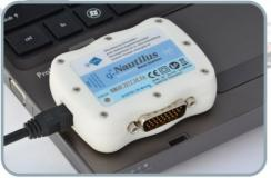
The g.Nautilus base-station connects directly to your PC/notebook via USB and does not require additional power. 8 digital trigger input channels allow the connection to various trigger sources to record precise timing information with the acquired signals.
